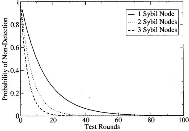
**Figure 1:** Probability of no Sybil nodes being detected, using the radio defense, with a channel for every neighbor. Assumes 15 neighbors (including Sybil nodes), any number of which could be malicious.
